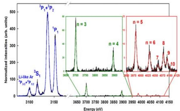
Fig. 1: X-ray transitions induced by the collision of 15 keV/q Ar<sup>17+</sup> ions with N<sub>2</sub> target.
