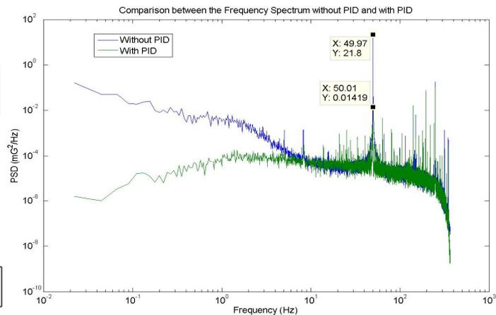
Figure 2 Noise spectral density before and after PID control
